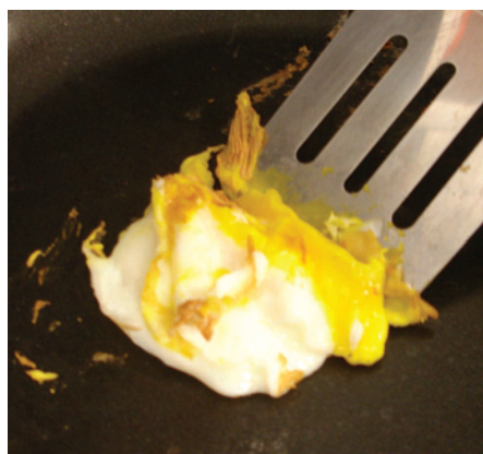
What egg failure looks like in the Dry-Egg Test (egg #34 on Nonstick "C").
